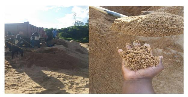
Sampling Mwogo sand against Mugonero sand to be taken to laboratory for testing in order to decide which sand to use in construction.
