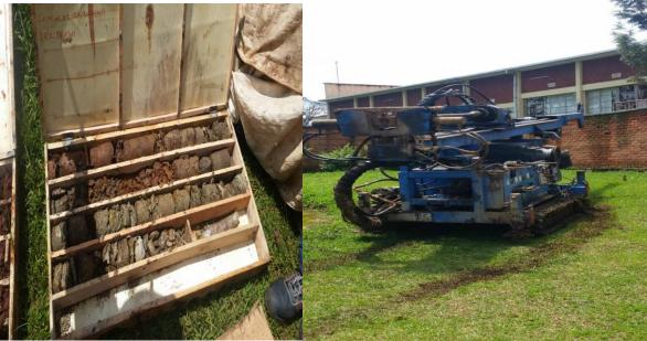
Photos: Sampling the soil for testing their bearing capacity.
