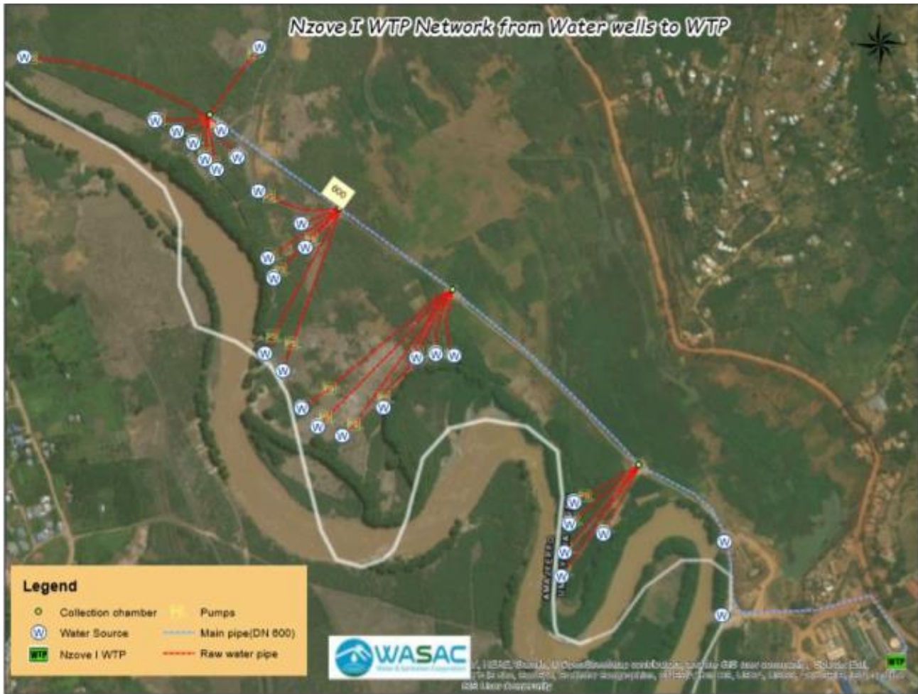
Figure: Groundwater collection pipeline (Red: Raw water pipe from each borehole to the raw water collection pipeline passing to the collection chamber)
